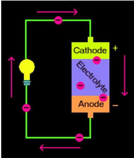
Olive: This picture shows a simple circuit of electrons flowing from the anode to the cathode. In the middle, we have another light bulb, and since the circuit is not broken, it is on.
