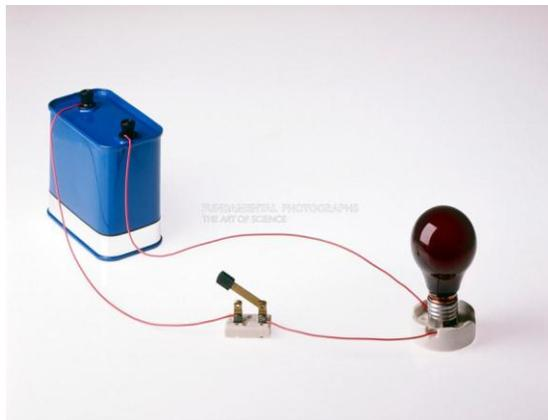
Here is a picture of a simple circuit. You can see the light bulb is not shining so we don't have a closed circuit. What could we do to get electricity to the light bulb?
